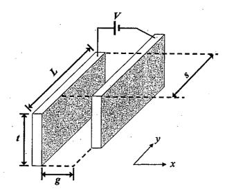
4. (30%) For the parallel-plate waveguide discontinuity in the figure below, find the power reflection coefficient for f = 7500 MHz for each of the following cases: (a) TEM mode; (b) TE<sub>1,0</sub> mode; and (c) TM<sub>1,0</sub> mode.
