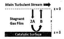
Please show that the molar flux of reactant through the film can be expressed as follows, where  $\delta$  is the effective gas-film thickness and  $x_{A0}$  is the molar fraction of A in the main stream. (8%)
